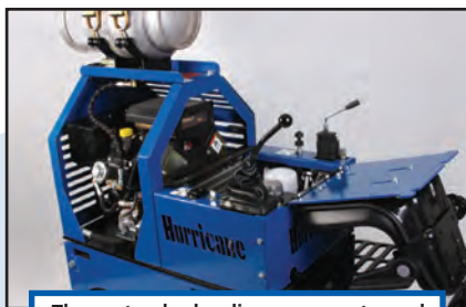
The motor, hydraulic components, and oil pressure gauge are easily accessible for simple maintenance procedures.
