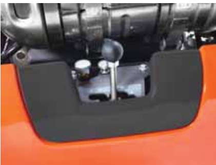
Located at the front of the saw, the gearbox shift lever is used to change the output speed of the engine gearbox. Three speeds and two neutral positions are standard. The gearbox shift lever positions (1, 2 and 3) are color coded to match the blade diameter and the bladeshaft rpm decal located on the control panel. Gearbox detant locks the gearbox shift lever in position.
