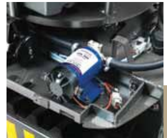
Electric filling pump.
