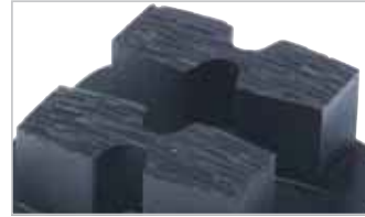
Husqvarna segment shape has more active diamonds than a basic rectangular shape. This means more aggressive grinding. They are pre-sharpened, enabling them to work with 100% efficiency at the start, without the need to dress the tool.
