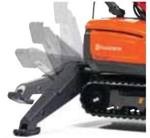
Outriggers with extra wide span for superior stability and high workload.
