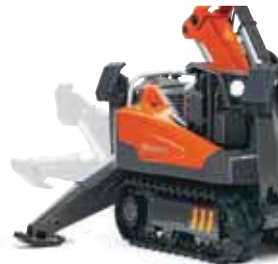
Individual control of the outriggers.
