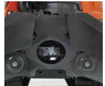
Release valve track tensioning.
