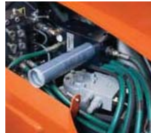
Grease pump, automatic greasing system is standard.
