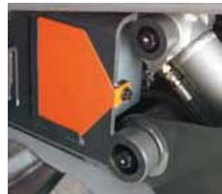
Release valve track tensioning.
