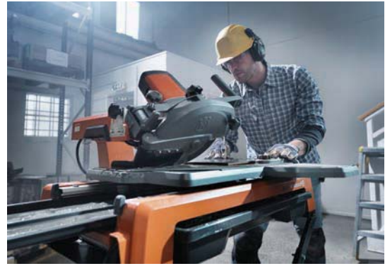
An extra long 26" conveyer cart supports larger tile.
