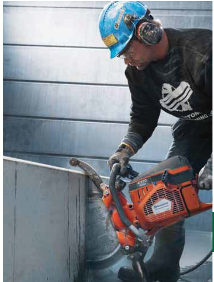
Cutting depth of 10", twice the depth of a traditional power cutter.
