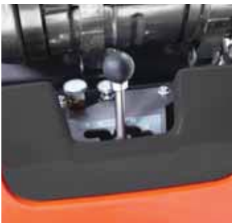
Located at the front of the saw, the gearbox shift lever is used to change the output speed of the engine gearbox. Three speeds and two neutral positions are standard. The gearbox shift lever positions (1, 2 and 3) are color coded to match the blade diameter and the bladeshaft rpm decal located on the control panel. Gearbox detant locks the gearbox shift lever in position.
