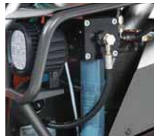
Grease pump and automatic greasing system for the tools is standard.
