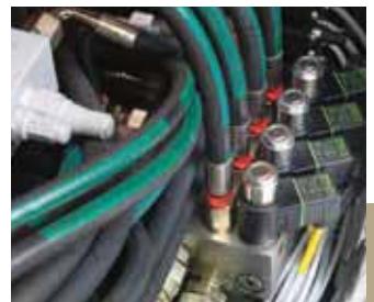
Plug-in. Attach/detach without tools.
