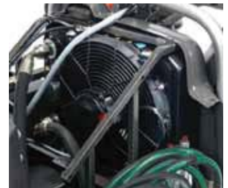
Automatic electric fan for extra efficient cooling.
