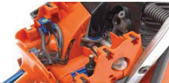
The heart of the OilGuard system is "the blue box". The fuel is led through the box where an LED shines through the fuel.
