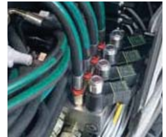
Plug-in. Attach/detach without tools.
