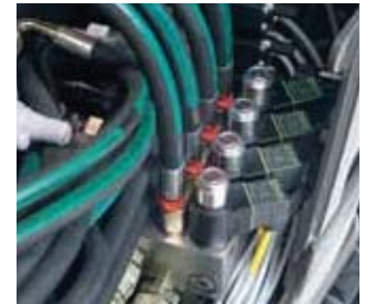
Plug-in. Attach/detach without tools.
