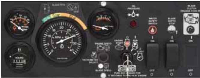
Tachometer/bladeshaft rpm gauge indicates engine rpm or bladeshaft rpm. Bladeshaft rpm range is color coded to gear selection position.
