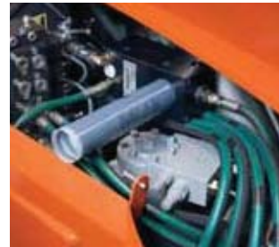
Grease pump, automatic greasing system is standard.
