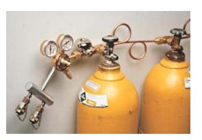
Air cylinders connected by tee blocks and pigtails, equipped with Audi-Larm Audible Alarm and air cylinder pressure regulator.
