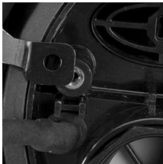
4. Align the upper tab to the screw holes in the upper lens ring.
