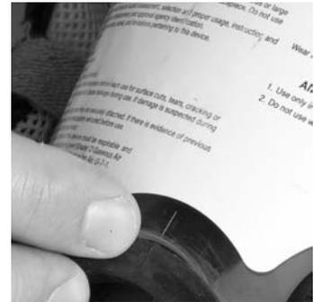
6. Moisten the mating surfaces of the facepiece and lens ring with Snoop (P/N 600920).
