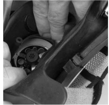
6. Route the microphone cable over the component housing retaining ring centerline.
