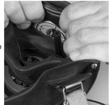
c. Stretch the nose cup over the retaining ring.
