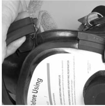
9. Press the ring halves together to mate the ends.
