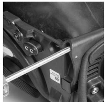
9. Use a Phillips screwdriver to tighten the component housing ring screw.
