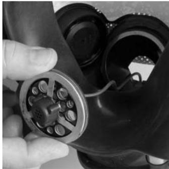
3. With the gasket forward place the microphone (P/N 10024076) into the component housing.
