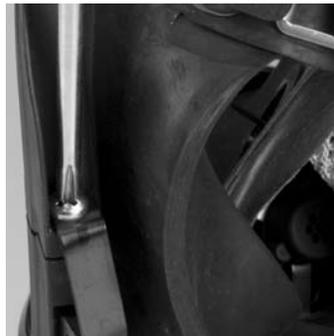
2. Use a Phillips screwdriver to remove the component housing ring screw.
