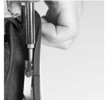
3. Align the screw hole in the lower metal tab with component housing screw hole.
