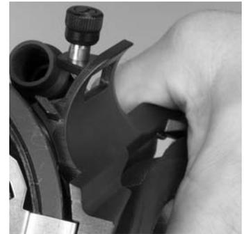
4. Reinstall the component housing cover. (See **Installing the Component Housing Cover** for instructions.)
