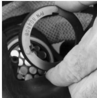
3. Carefully remove the speaking diaphragm.
