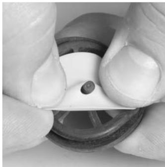
2. Insert the gasket so that the groove captures the housing rim.
