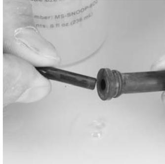
2. Lubricate the barb with Snoop (P/N 600920) and push the drinking tube onto the drinking tube connector 1/2".
