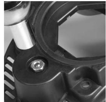
c. Use the **Pneumatic Nut Special Tool** (P/N 10086032) and a 1/4" socket to remove the pneumatic nut.
