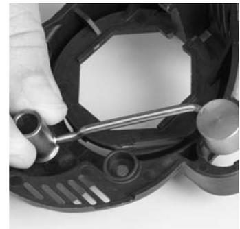
**Note:** The pneumatic assembly nests easily in the component housing. Take care not to bend or flex the tube when installing the pneumatic assembly.
