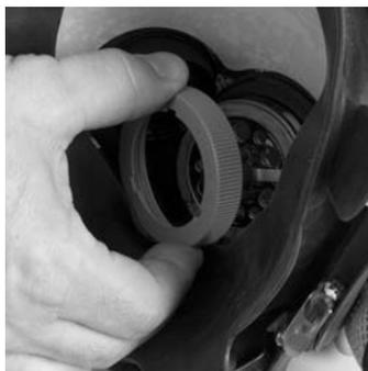
4. Install the retaining ring (P/N 10023505) and firmly hand tighten.
