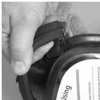
3. Pull the lens out of the groove.
