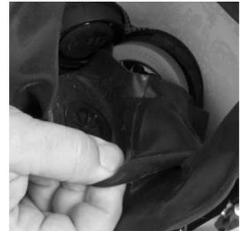
7. Unscrew and remove the speaking diaphragm retaining ring.
