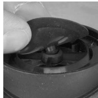
2. Ensure that the nosecup does not interfere with valve disc operation.
