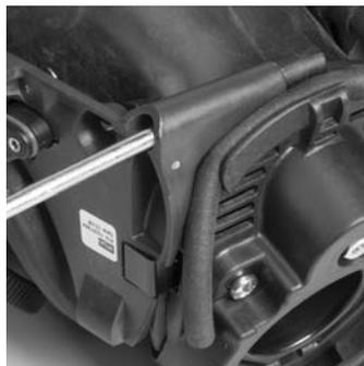
3. Remove the component housing cover. (See **Removing the Component Housing Cover** for instructions.)
