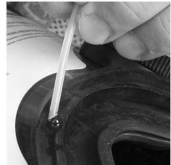
7. Lubricate the lens ring with Snoop (P/N 600920).
