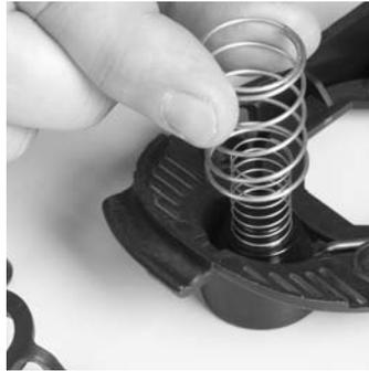
c. Remove the pneumatic spring.
