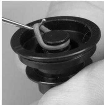
f. Use the o-ring removal tool to remove the o-ring.
