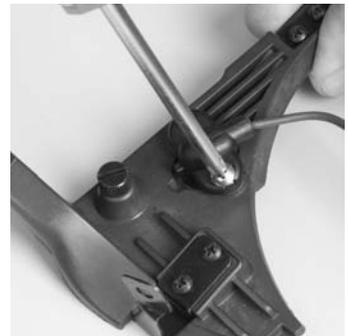
8. Use a small Phillips screwdriver to connect the ClearCommand microphone to the mounting bracket.
