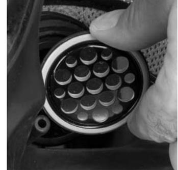
2. Install the retaining ring (P/N 804808) and firmly hand tighten.
