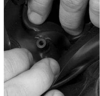
b. Stretch the nose cup over the exhalation valve flange.
