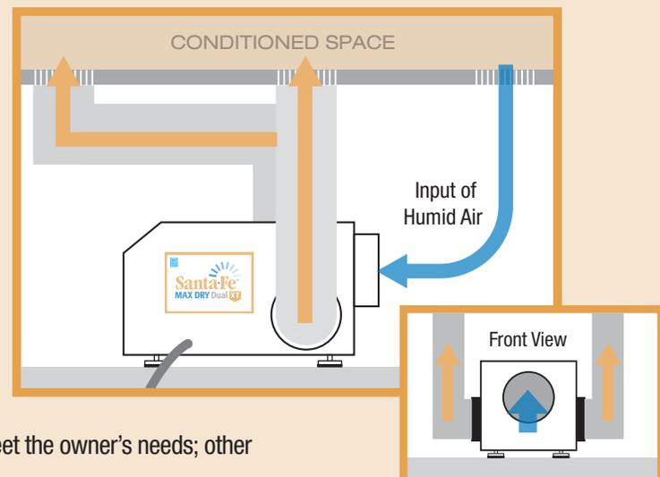
The Santa Fe Max Dry Dual XT can be installed in a variety of locations to meet the owner's needs; other considerations include:
