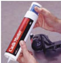
2. Drop in new cartridge and twist barrel to lock.
