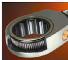
The box end ring gear has 72 extra-fine teeth, allowing the ratchet mechanism to engage with just a 5° movement of the wrench. This important component is pre-precision machined and specially heat-treated for exceptional strength.
