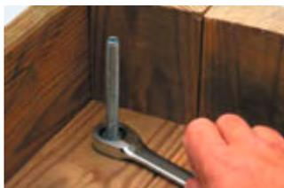
Works in places even deep sockets won't reach. It's the perfect tool for positioning and tightening bolts on threaded rod adjusters like those found on most electric garage door openers.
