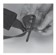
d. Pass the first stage intermediate-pressure hose through the tunnel.
