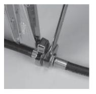
a. Use a torque wrench with 11/16" crowfoot to tighten the connector to 125 ± 5 in lbs.
