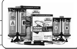
Handi-Foam® Quick Cure Spray Foam is a low pressure foam system that utilizes a non-flammable blowing agent. Handi-Foam Quick Cure Spray Foam has been specifically formulated for flame retardancy and conforms to the requirements of ASTM E84 as a "Class 2(B)" system (flame spread of 75 or less, smoke development of 450 or less). The foam helps to lower heating and cooling costs by drastically reducing energy consumption.
