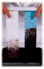
Spilfyter's fine fibers enable superior wicking versus coarse fiber products. In an 8-hour Vertical Wicking Test, Spilfyter absorbed 133% more liquid than coarse fiber products!
