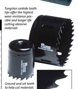
3 teeth per inch creates wider gullet for better chip clearance and faster cutting
