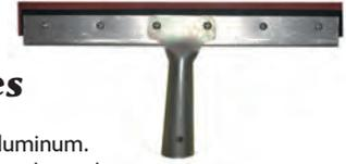
Frame is made of heavy gauge aluminum. Handle socket is cadmium-plated steel. Double squeegee rubbers. Squeegee rubber is red. Back-up rubber is black.
