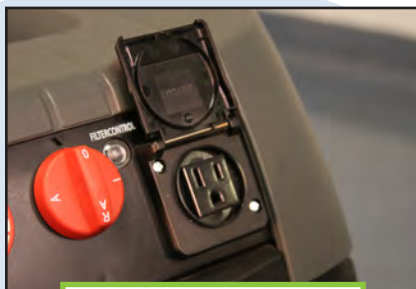
Simple control panel with auxiliary outlet for hand tools.
