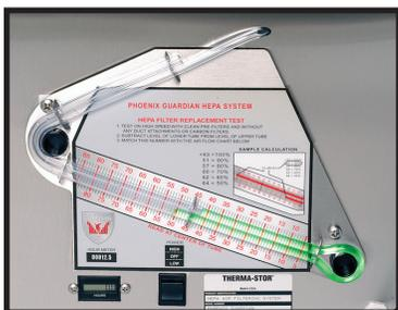
The built-in manometer provides precise measurement of air-flow through the HEPA filter and aids in determination of HEPA filter replacement intervals.
