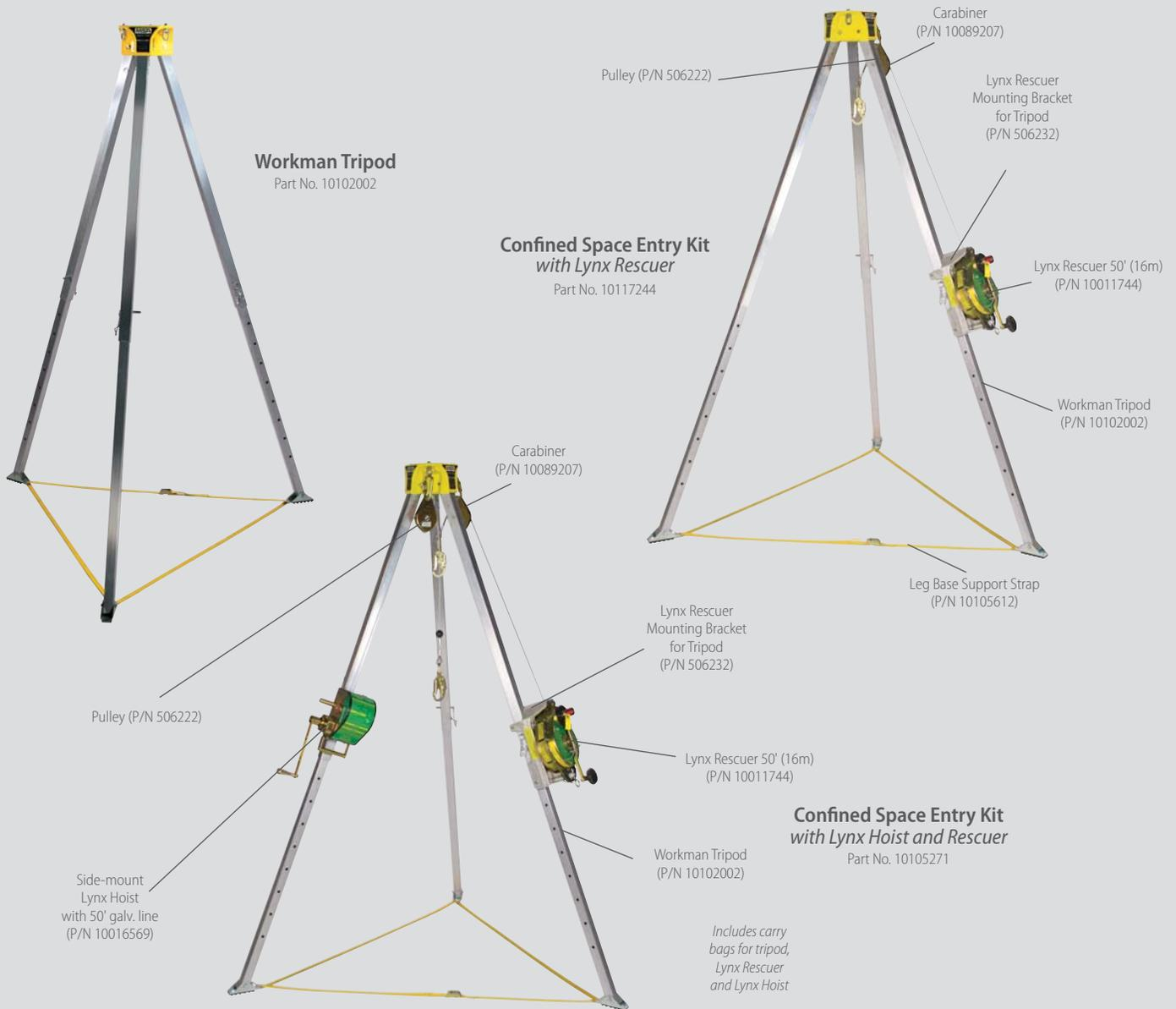
MSA Tripods make confined space entry with vertical descent easy. The Workman Tripod features an internal leg-locking mechanism, a maximum height indicator on the tripod legs, cut-resistant leg pin retention chains, recessed product labels, a reduced weight and an integral carrying strap. The Workman Tripod can be set up and dismantled without the use of tools.
