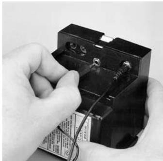
**Note:** To use the dual-rate charger, insert the charging plug in the charging jack as usual. Then insert the male control plug into the center jack in the battery pack.
