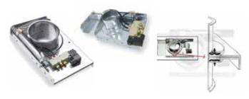
Truly "air-tight" blast gates operate manually or pneumatically and utilize a two part, self-sealing gasket assembly to completely isolate outside air, guaranteeing no air leakage across the valve or into the atmosphere. Designed to withstand 16 Hg" of negative pressure. Available in Zinc Plate or Stainless Steel.
