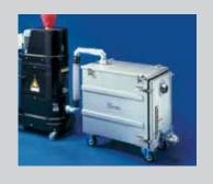
For over 30 years Ruwac's portable immersion separation systems have been safely collecting aluminum, titanium and other Group E explosive dusts or glowing media. With 100% of the intake air being completely submerged in turbulent liquids, the chance of an outside ignition source entering the vacuum is safely ruled out. Contact us today with your specific application to see if an immersion separator may be your solution.
