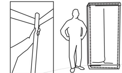
4. Position and tension the poles into the corners in the recessed slots on the base and top panels.
