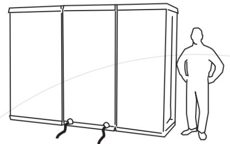
6. For D-Con 3 and D-Con Blue, repeat assembly instructions for the shower unit, note the sump on the standard D-Con has a elevated plastic and foam platform to keep the worker out of the drain water. D-Con 3 and D-Con Blue both have a shower unit with blue water supply and drain ports at the base. Position the system with shower so that the blue water supply and drain ports face the adjacent water source and pump. For D-Con 2, skip #8, no shower is included.
