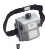
HEPA PAPR Assembly 231-01-30 Includes: Air Filter Unit 520-03-63R01 HEPA Filter 451-02-01R01 Belt 021-41-02R01 Airflow Indicator 021-14-00R01
