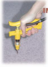
Injectimate allows you to mix your solution in a gallon container and to inject directly from the container without having to fill a syringe. Every squeeze of the unit automatically injects 5 milliliters of solution.
